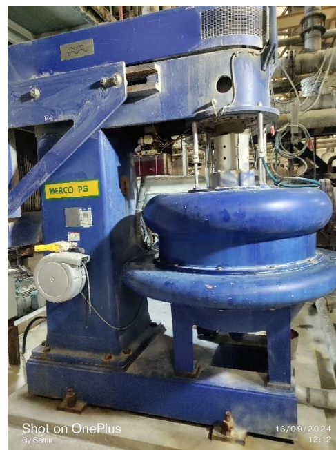
Germ Separator – Alfa Laval Nozzle Centrifuge
